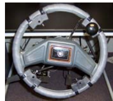
Steering wheel – From a 1987 Cadillac Deville, with full telescoping and tilt functionality.
